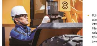
Uptime has been increased by extending the standard service interval for the oil and oil filter to 500 hours, which also reduces maintenance costs, and by adding an optional autogrease system.
