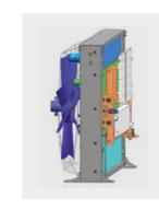
The HL940A has a dependable wide-core and fin air cooler that prevents performance degradation caused by contamination. It is also equipped with a reversible fan to eliminate dust and debris. A turbo pre-cleaner is available as an option to further extend the replacement cycle.
