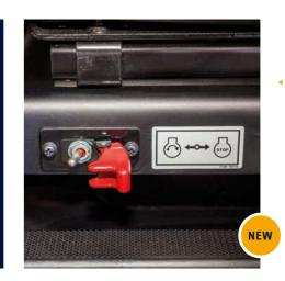
**Emergency stop switch** The engine can be shut down immediately using an emergency stop switch located at the base
