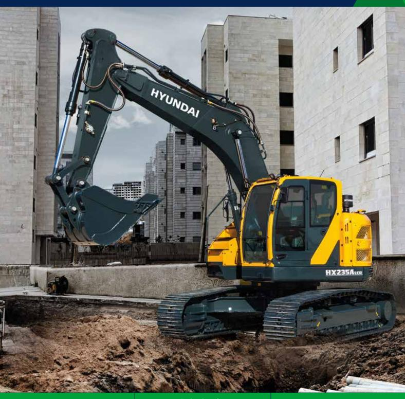
Gross Power 129 kW (173 hp) at 2200 rpm Bucket Capacity 0.70 ~ 1.05 m<sup>3</sup> Operating Weight 17170 kg & 18820 kg
